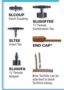
\*End Cap can be made from Techline CV, Techline or 17mm Techlite Dripperline by folding 8mm Techlite tubing over twice and sliding 1<sup>1</sup>/4" cut section over the end.
